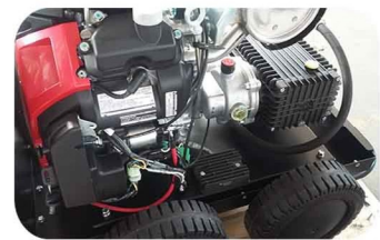
ENGINE-PUMP COUPLING using reduction gear.
